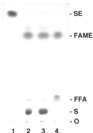
FIG. 1. Identification of reaction products by TLC. Cholesteryl oleate was incubated with a mixture of methyl propionate and 0.84 M NaOH in methanol (2:3) at 37°C for 1 h (lane 2). Cholesteryl oleate was also developed on a silica gel TLC plate in hexane/acetone (96:4). After visualization with 0.01% primuline in methanol, the corresponding band was scraped off into a vial. The cholesteryl oleate was methylated in the presence of silica gel by a similar procedure with minor modifications (lane 3). The pale spot found between SE and FAME in lane 2 or lane 3 is cholesteryl propionate. Lane 1, cholesteryl oleate (before reaction); lane 4, authentic lipids (FAME and FFA). Developing solvent, hexane/ tert -butyl methyl ether/ acetic acid (85:15:0.5). SE, sterol ester (cholesteryl oleate); S, sterol (cholesterol); O, origin.
